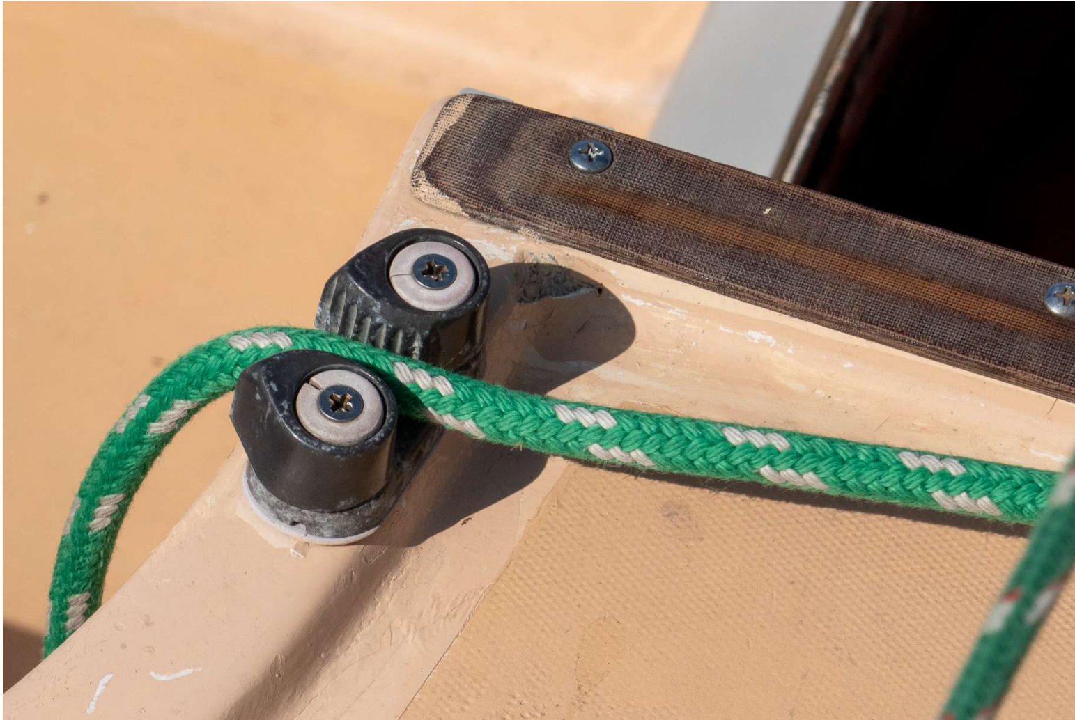
cleat for Victory jib sheet (cam cleat)
